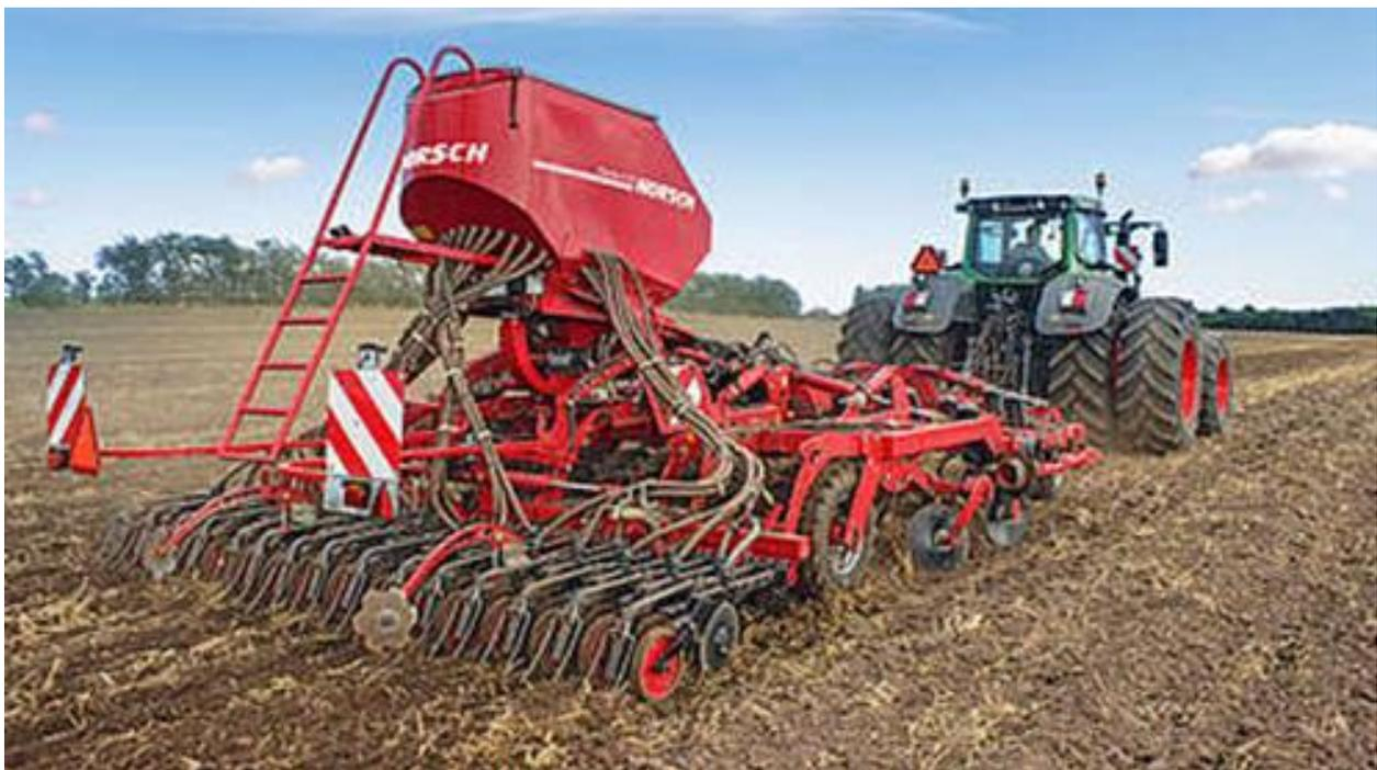
*The seed harrow forms a plain surface on the cultivated area, but if there are poorly chopped crop residues, straw heaps can be dragged together.*
