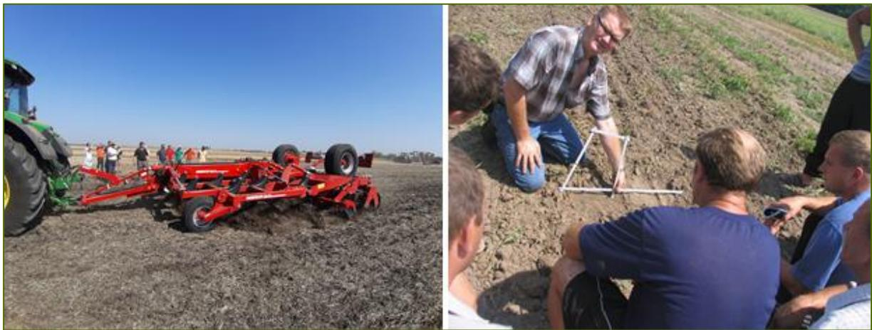
*Tillage depths of 3.5 to 4.5 cm are possible with the compact disc harrow, every cm means that approx. 150 t per ha more soil have to be moved, which can then also dry out.*
